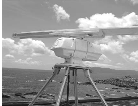
Fig. 5 Fixed coastal radar monitoring system
