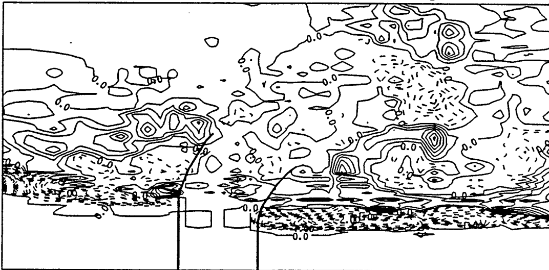
Bathymetric Change Contours of S8 after 6-Day(NE) Storm
