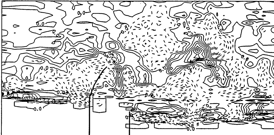
Bathymetric Change Contours of S0 after 6-Day(NE)Storm
