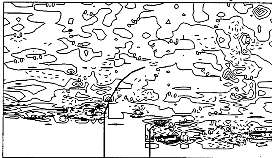
Bathymetric Change Contours of S2 after 8-Day Recovery
