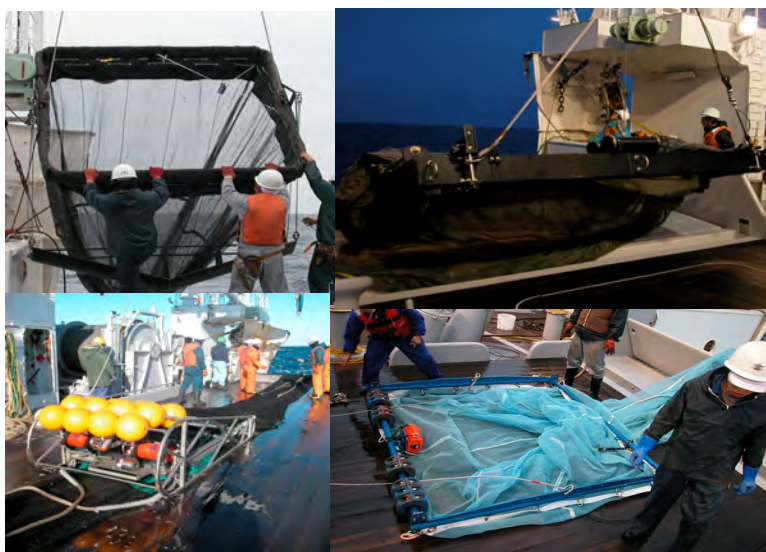
Fig. 1 Comparison of sampling gears during the MIE-2 cruise: MOHT (left top), MOCNESS-10 (right top), rope trawl with multi-sampler (left bottom), and HUFT (right bottom).
