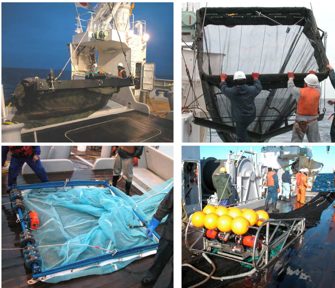
Fig. 3.3 Sampling gears tested during the MIE-2. Upper left: MOCNESS-10, upper right: MOHT, lower left: FMT (= HUFT, with fine mesh net), lower right: otter trawl (OT) + Multisampler.
