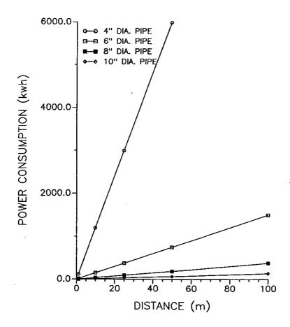
Figure 2. Power consumption (kwh) vs. distance (m) for various pipe diameters.
