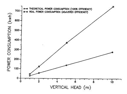
Figure 1. Theoretical and real power consumption (kwh) vs. vertical head.
