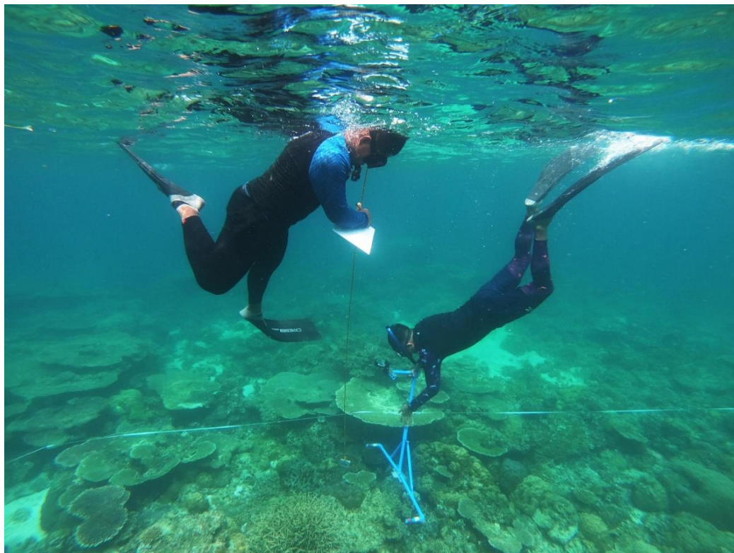
Figure 3. The navigator (left) and photographer (right) researchers while photo-documenting the substrate using the C30 method.
